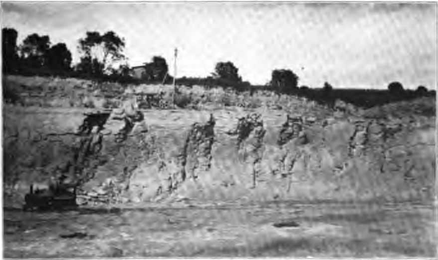
B.—View of the shale pit of the Medal Paving Brick Company near Wooster. Shale of the Black Hand member passes into sandstone near the top of the quarry face.
